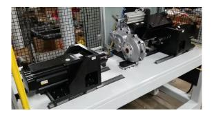
Signalysis is working with Farris Automated Systems on a custom gearbox tester for golf carts. The machine uses a non-contact vibration sensor that's so accurate, it not only tells what gear has the problem, but it can tell you what tooth has the problem.
