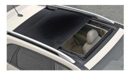
The Signalysis Sunroof Test System is designed to handle complex & dynamic noise issues associated with power sunroofs and roll shades. Using motor current and hall effect sensor counts a detailed motion/location event matrix is created that encapsulates customer complaints. This matrix allows unique GO/NO GO metrics to be developed which will result in high customer satisfaction ratings.
